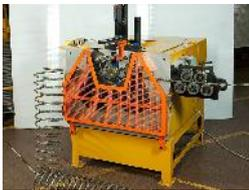
Particularly suitable to process long spirals and micropales. The 88 can execute spirals and hoops with a minimal diameter of 140 mm up to 600 mm with its standard tools and with the fitting of a special tool, diameters up to 1500 mm.
