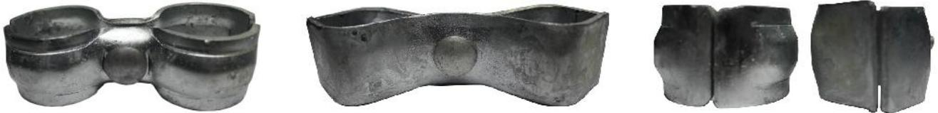
An example of how additional strength was obtained by having pressed deformations in the design of the clamp was highlighted in the test results of the five 4040 clamps. The force applied to these clamps to achieve a fail rate varied from 350 kgs to 700 kgs. The fitting without pressed deformations required much less force before it failed than the clamp having well-formed deformations. The metal thickness of all 4040 clamps only varied from 3.8mm to 4.1mm.
