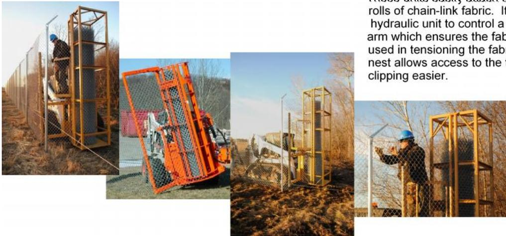
These units easily attach to a Bobcat, and hold 30 metre rolls of chain-link fabric. It comes equipped with a hydraulic unit to control a side kickout and stretching arm which ensures the fabric remains level. The arm is used in tensioning the fabric to an end post. A crow's nest allows access to the top of the fencing roll making clipping easier.
