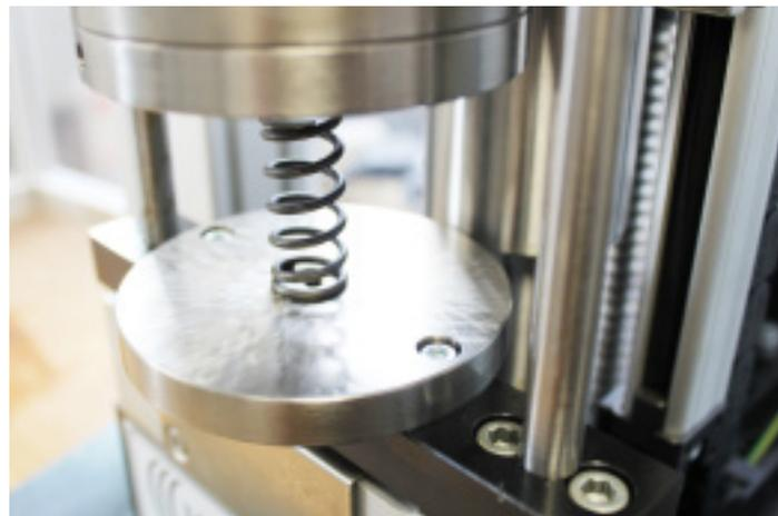
Although more complicated and costly, the benefits in general far outweigh the negatives regarding prestressing. Prestressing not only stabilises the dimensions of the spring, leading to a more predictable product during operation, but also allows the spring to work to higher stresses. Working under higher stresses, springs are more optimised, making them significantly lighter and can save on material costs.
